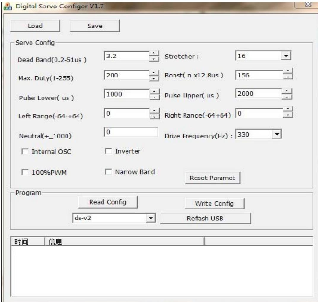
5. Click “Reflash USB”, the information column will show “找到设备(device is found)”, it means the software can be programmed now.
